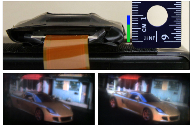
Figure 3: The OLED-based prototype. (Top) A modified eyepiece is shown in profile. The ruler illustrates a thickness of 1 cm. The microlens array (length shaded blue) is thinner than the OLED enclosure (length shaded green). (Bottom) A stereoscopic pair of photographs of the binocular prototype. The left-eye and right-eye images are interchanged to facilitate cross-fused stereo viewing.
